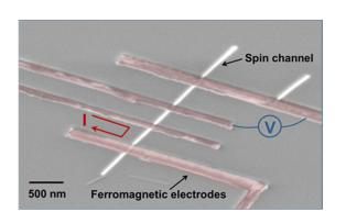
SEM image of a spin-valve device in which the charge and spin currents are separated (Courtesy of Dr. Marius Costache, ICN2).
