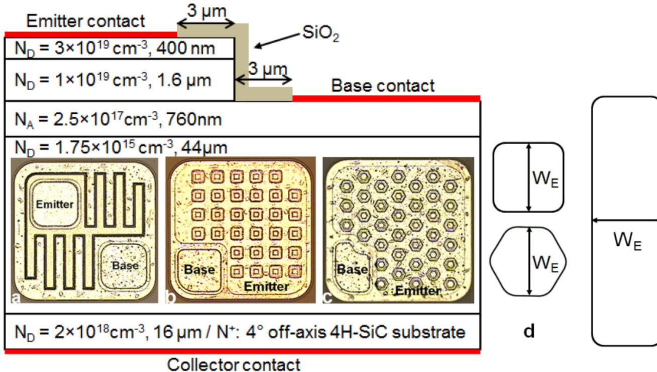
At the first time, new cell geometries (square and hexagon) were investigated for BJTs, which opens a new design space for improved performance.
