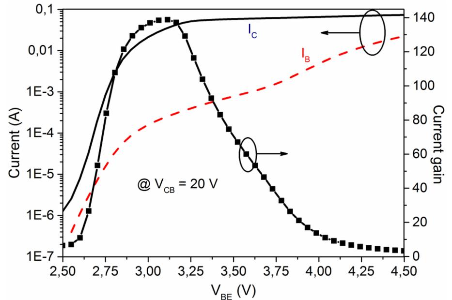
A current gain record of **139** for 15 kV-class BJTs
