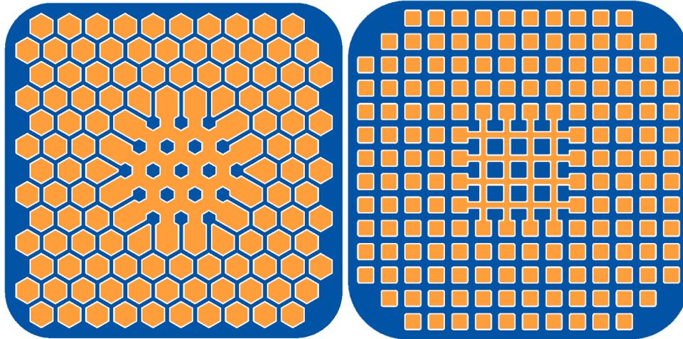
The hexagon and square emitter contacts (orange) and base contacts (blue) which are inverted in the center of BJTs to form the intertwined design.
