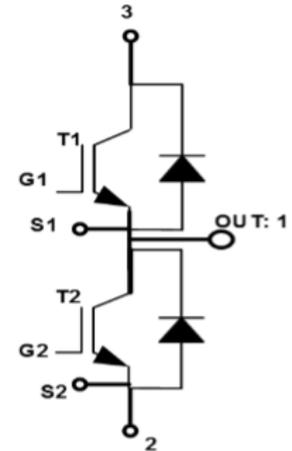
$V_{CES} = 1700 \text{ V}$ ,  $I_{CE} = 300 \text{ A @ } 25 \text{ }^\circ\text{C}$
