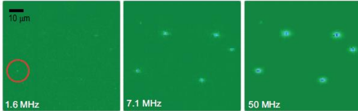
Figure 4.3: Spatial maps of the measured capacitance change ( \Delta C_{\text{exp}} ) induced by the sedimentation of insulating 4.4- \mu\text{m} -radius particles at a salt concentration of 150 mM for frequencies of 1.6 MHz, 7.1MHz and 50MHz. Each pixel represents a nanoelectrode and each map was normalized to the maximum value of |\Delta C_{\text{exp}}| over all the three pictures. The sensitivity to the presence of microparticles increases with increasing frequency.
